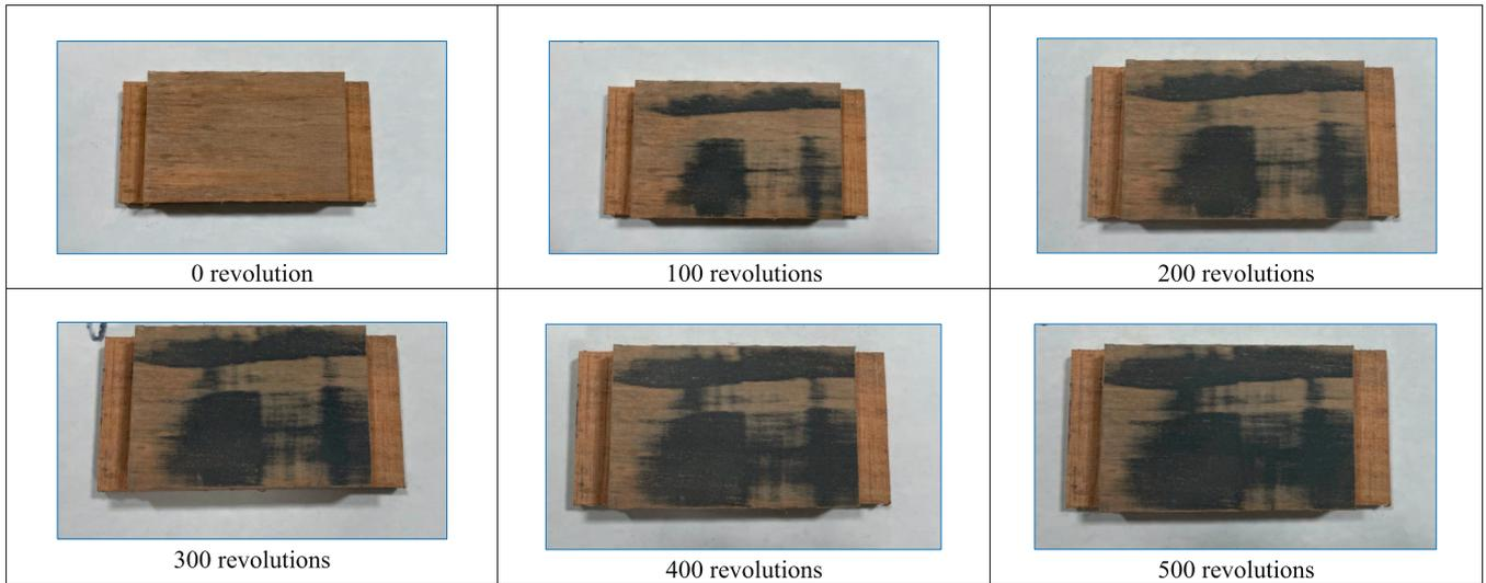
Figure 1.—Sweetgum control (undensified) specimens after different revolutions by Navy-Type Wear Tester.
