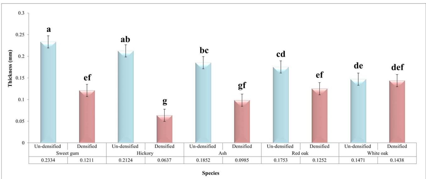
Figure 2.—Thickness loss of control (undensified) and densified of five hardwood species Materials with the same letter were not statistically different from each other at the  $\alpha = 0.05$  level of significance.
