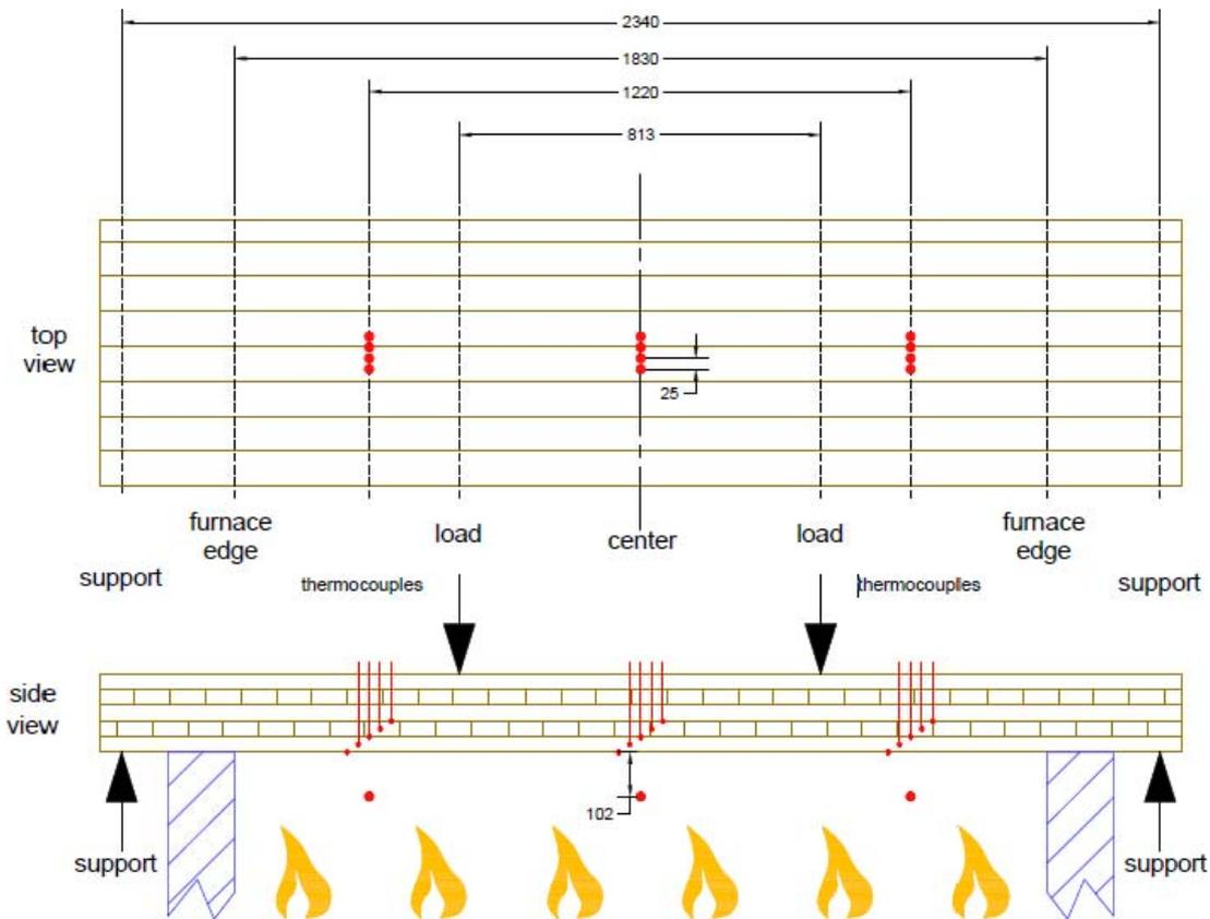
Figure 1.—Panel layout and thermocouple locations (distances given in millimeters).
