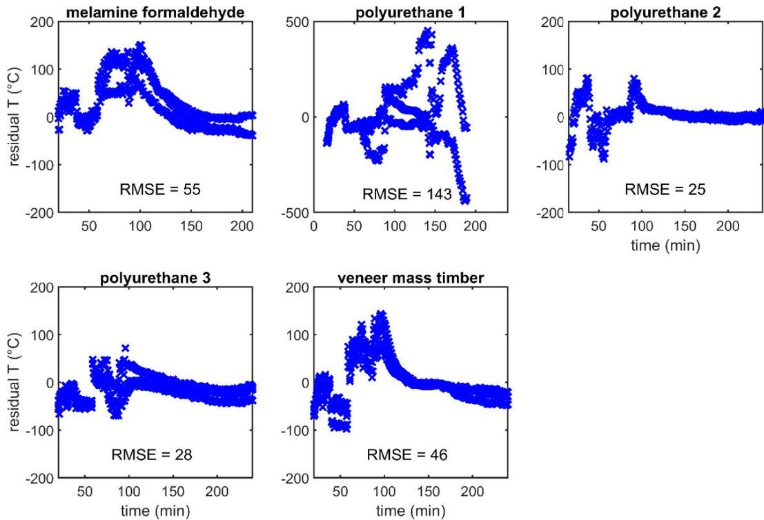
Figure 6.—Temperature residuals (intermediate test – full-scale test data) along with the root mean square error (RMSE; units degrees Celsius) for the different panels tested.
