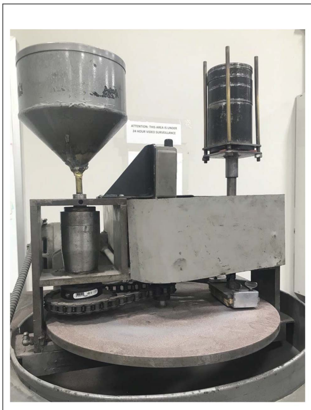
Figure 2.—Navy-type wear tester used to conduct abrasion test.
