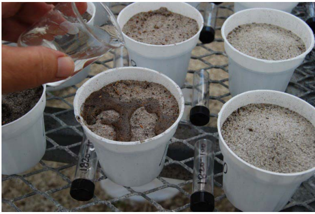
Fig. 3. Example of irrigation water beading on the surface of HSP substrate (hydrophobic 90:10% v/v sand:peat).
