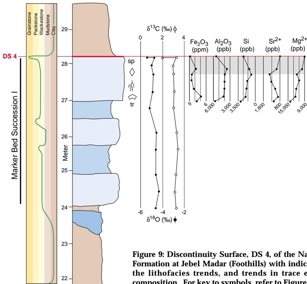
**Figure 9: Discontinuity Surface, DS 4, of the Nahr Umr Formation at Jebel Madar (Foothills) with indication of the lithofacies trends, and trends in trace element composition. For key to symbols, refer to Figure 4.**
