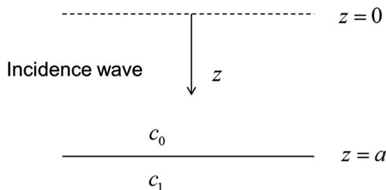
**Figure B-1.** A 1D acoustic model with velocities  $c_0$  over  $c_1$ .
