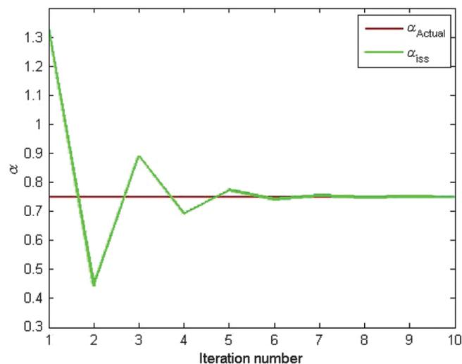
**Figure B-5.** The estimated  $\alpha$  at  $R = 0.3333$ : The horizontal axis is the order of the ISS subseries, and the vertical axis represents the value of  $\alpha$ . The red line shows the actual value of  $\alpha = 0.7500$ . The green line shows the estimation of  $\alpha$  using the ISS inversion method order by order.
