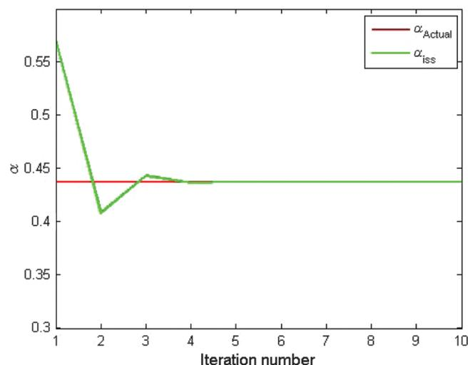
**Figure B-2.** The estimated  $\alpha$  at  $R = 0.1429$ : The horizontal axis is the order of the ISS subseries and the vertical axis shows the value of  $\alpha$ . The red line shows the actual value of  $\alpha = 0.4375$ . The green line shows the estimation of  $\alpha$  using the ISS inversion method order by order.
