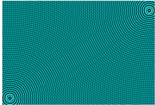
Figure 2. Simulation from rippletank app, [www.falstad.com](http://www.falstad.com). Point sources bottom left, top right, around 80 wavelengths apart. Elliptical standing waves are visible.
