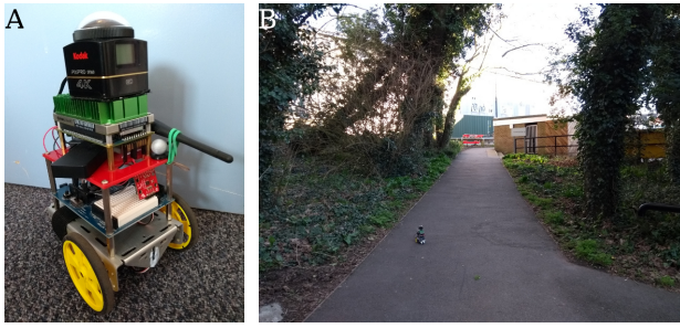
Figure 1: A Robot platform with onboard computation. B Environment used for robot testing.
