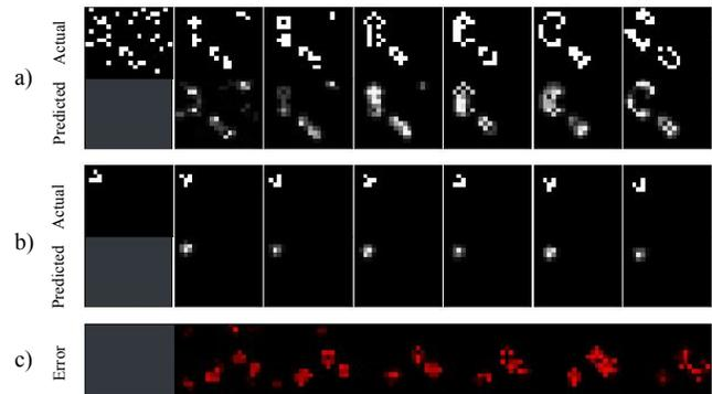
Figure 9: **Predictions with smaller convolutional filters.** The settings are the same as for Fig. 5, but the filter size is  $2 \times 2$  instead of  $3 \times 3$ . (a) Predictions from a random initial state. (b) Predictions for a initial state composed of one glider. (c) The difference between actual and predicted images. The performance is poor. The filters are too small to capture neighborhood information.
