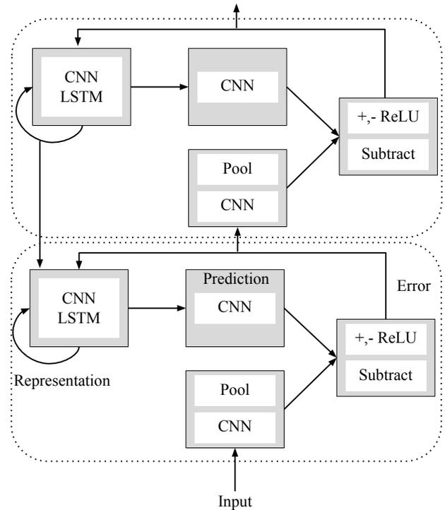
Figure 1: **The architecture of PredNet.** Figure modified from Lotter et al. (2016). The network is divided in modules (solid lines) that are stacked into layers (dashed lines). The input to the first layer is the original image frame at  $t$ ; the error between the prediction at  $t$  and the frame at  $t + 1$  is passed as input to the next layer. There are 3 layers in total (only 2 represented here.)
