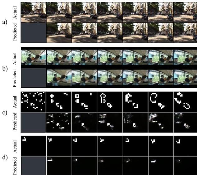
Figure 2: **Predictions generated by a PredNet trained on the KITTI dataset.** See Table 1 for measured performance. (a) Predictions for KITTI, the original training dataset. The performance is high. (b) Predictions for the FPSI dataset. The performance is also high. (c) Predictions for a random initial value of the GoL. The performance is poor, as expected. (d) Predictions for a GoL glider. The performance is also poor.
