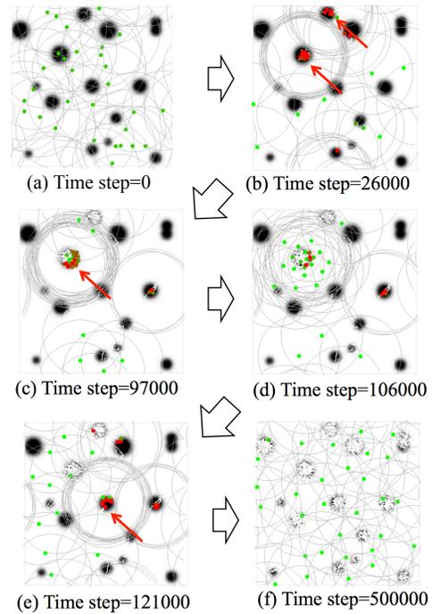
Figure 1: Simulation result. Areas in which  $V(\mathbf{r}_i)$  is large are denoted by a dense color. Agents with high and low workload are colored by red and green, respectively. Gray circles denote the sensor range of the agents. The meanings of the red arrows are explained in the main text.
