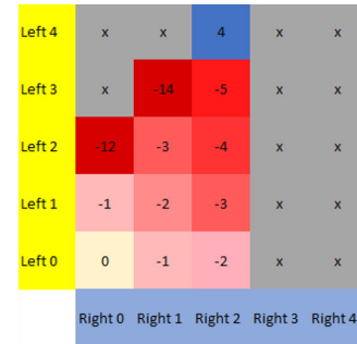
Figure 3: The fitness landscape of all 25 possible agent solutions in the RC- environment, where there is a cost of -1 per move. The 13 invalid solutions are indicated with an ‘x’, whereas the 12 valid solutions show the fitness received if the agent moves the specified amounts to the right then left (i.e. 2 moves right then 4 left gives a fitness of +4, after a movement penalty of -6 ). Rewards and penalties are the same as in Figure 2, with an additional cost to movement.
