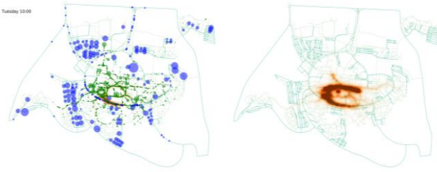
Figure 2: Agent-based simulation of pedestrian traffic on the Binghamton University campus. Left: Visualization of agent movements (green dots: individual agents; blue dots: vehicles; green discs: indoor space occupancies; blue discs: parking lot occupancies). Right: Heatmap showing the simulated density of close contact incidents. See (Sayama & Cao, 2020) for more details.
