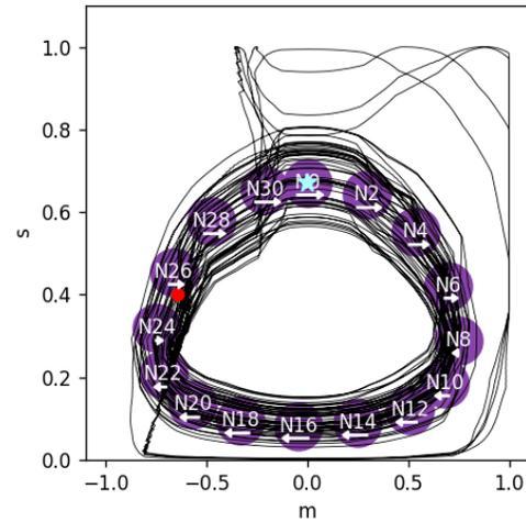
Figure 1: Node positions and sensorimotor trajectory of the robot in Exp. 2. Arrows indicate the  $N_{VA}$  values for each node at end of training. The blue star shows the sensorimotor state at the end of the training phase, and the red circle shows the sensorimotor state at the end of the trial.
