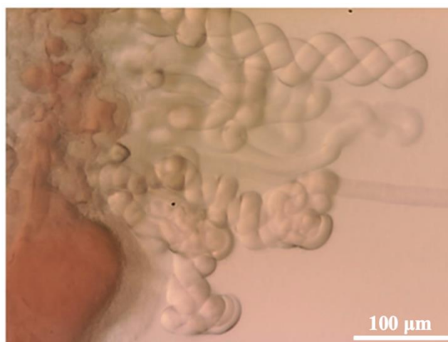
Figure 6: Examples of helical myelin figures observed by optical microscopy. Initial conditions: decanol droplet placed over an aqueous solution of 10mM sodium decanoate and 1mM KCl at basic pH.
