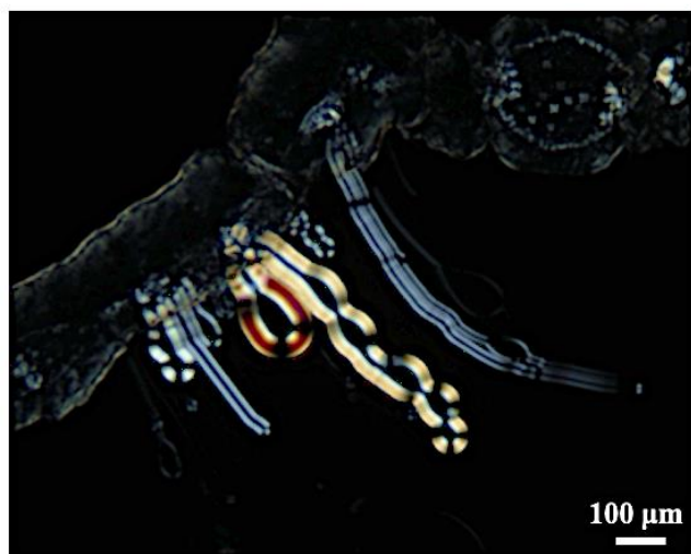
Figure 5: Examples of myelin figures observed by polarized optical microscopy. Initial conditions: decanol droplet placed over an aqueous solution of 10mM sodium decanoate and 1mM NaCl at basic pH.
