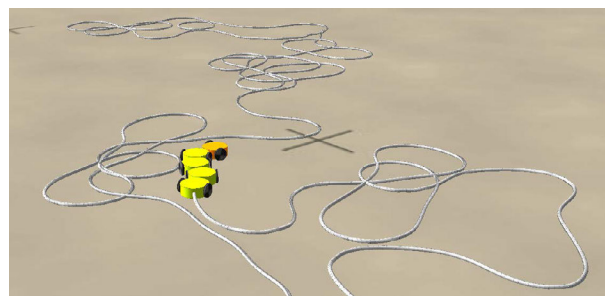
Figure 4: A train consisting of elastically coupled cars. The attractor resulting from a projection to a reduced phase space is manifestly not a limit cycle.
