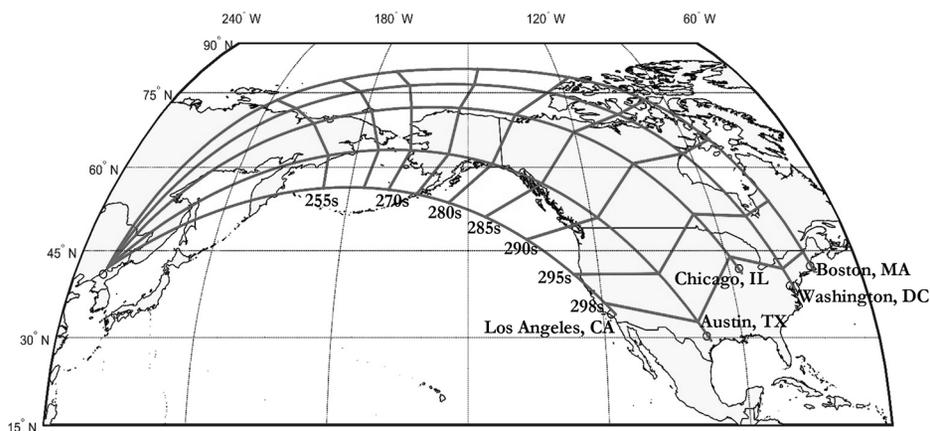
NOTE: The launch site for this ICBM is from the northwestern launch site near Chunggangup. The time contours across the trajectories denote the impact point of the missile payload if interception occurs at that time in the missile's boost-phase.
