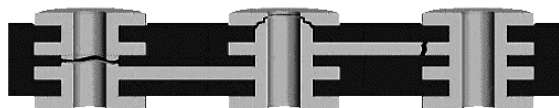
Figure 1: PTH failures. Barrel fracture, shoulder fracture and inner layer separation (from left to right)
