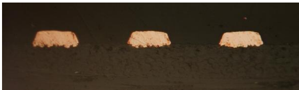
Figure 4. Comparison of Profile-Free Copper on X-R-1 Laminate (Upper) And High Tg Epoxy Laminate (Lower).
