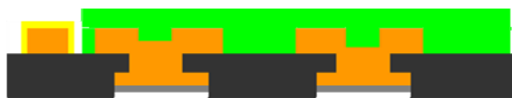
Fig. 3: Schematic of aS 3 (singled sided substrate) substrate based on coreless process flow.
