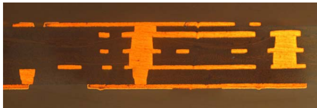
Fig. 8: Partial cross-section of 5 layer coreless organic substrate.
