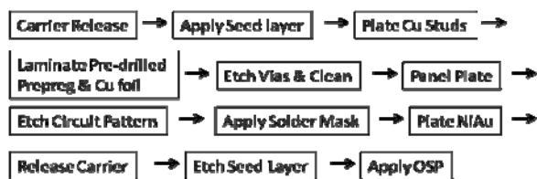
Fig. 4: Schematic of process flow for aS 3 type substrate.
