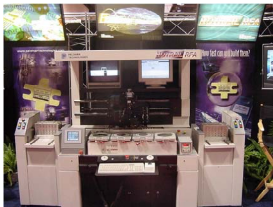
Figure 9 – Automatic Magazine to Magazine Header Load/Unload and 4 Wafer Frame/Grip Ring RFSOE Eutectic Assembly Cell
