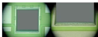
Figure 12 – Large Die Eutectic Attachment
