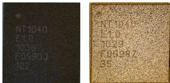
Fig. 7 Examples of non-plated and shielded parts.
