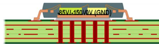
Figure 3: Test vehicle for investigation of ink-jetting for die attach with two chips arranged side by side in a quad flat package type.
