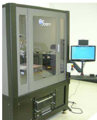
Figure 5 - nScript 3Dn-450 direct printing equipment
