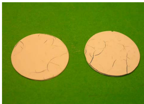
Figure 9: Sandwich specimen of NEB20/DuPont 951 laminated using a uniaxial press followed by room temperature isostatic pressing and co-firing at 850°C for 0.5 hours.
