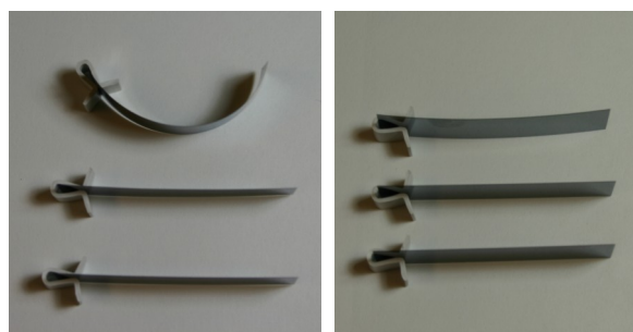
Figure 3: Bending of silicon test pieces due to film stress. Left: 50 micron silicon test pieces. Right: 100 micron silicon test pieces.
