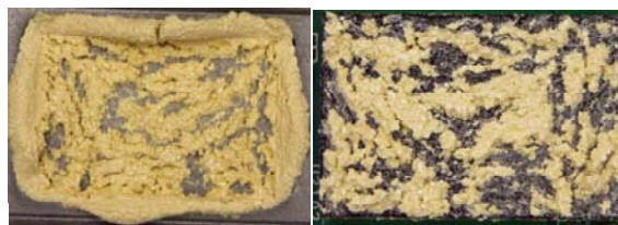
Figure 15: Photos of heat spreader (N9) location (left) and module (right) after thermal cycle test, without any copper electrode. No evidence of TIM pumping.
