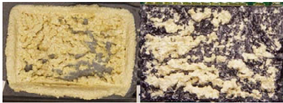
Figure 16: Photos of heat spreader (N9) location (left) and module (right) after power cycle test, without copper electrodes. No evidence of pumping.
