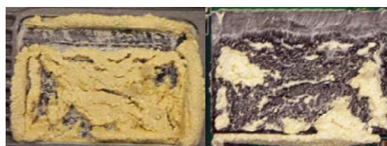
Figure 14: Photos of smooth heat spreader location (left) and module (right) after thermal cycle test, without any copper electrode. Evidence of TIM pumping is present; ~20% loss in TIM area.
