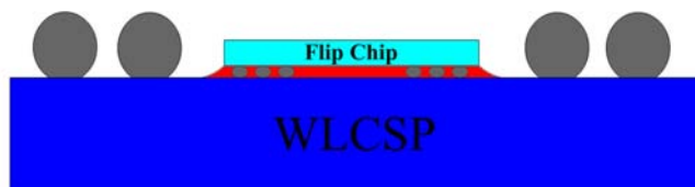
Figure 1. The Schematic View of 3D-WLCSP Technology: Flip Chip Silicon to Silicon Wafer Level Integration
