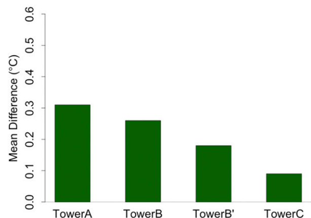
FIG. 4. Tower A (4 m), tower B (30 m), tower B' (50 m), and tower C (124 m) mean air temperature difference computed with respect to tower D (309 m) for aspirated PRTs.
