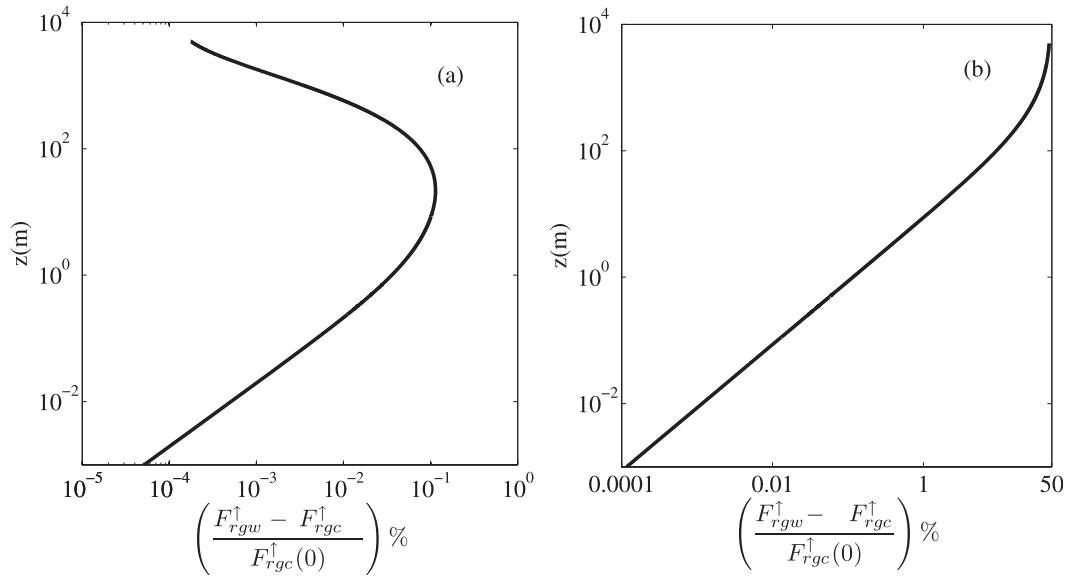
FIG. 2. Differences in the erroneous and correct reflected fluxes (normalized by the reflected flux at the surface in the particular band) for a tropical atmosphere and for the frequency ranges (a) 1550–1650  $\text{cm}^{-1}$  (the 6.3- $\mu\text{m}$  vibration–rotation band) and (b) 720–800  $\text{cm}^{-1}$ ; the band-averaged transmittance is given by (11) with the band parameters taken from Rodgers and Walshaw (1966).
