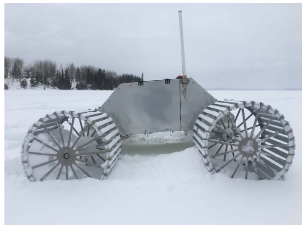
Fig. 5 Side view of FrostyBoy after becoming immobilized
