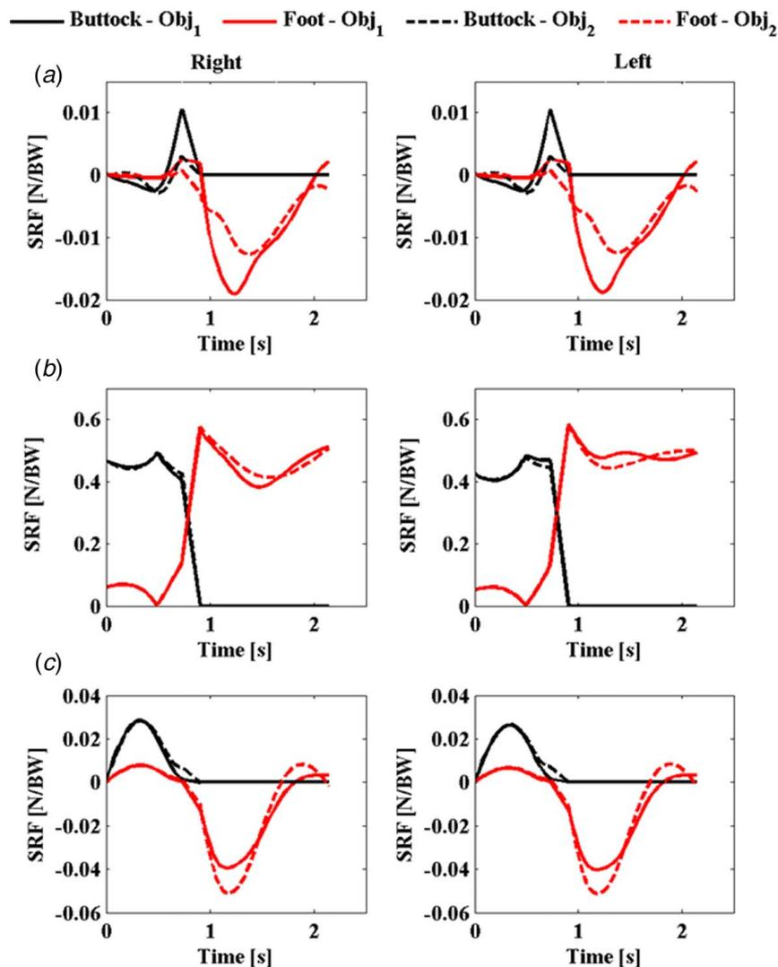
**Fig. 7** SRF profiles of a healthy elderly virtual-individual during an assisted STS maneuver: (a) M/L, (b) vertical, and (c) A/P
