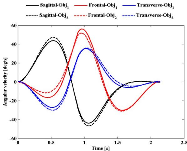
**Fig. 5** Upper-body joint velocity profiles of a healthy elderly individual during an assisted STS task
