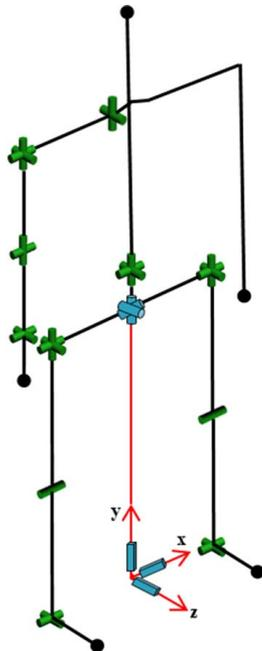
Fig. 1 30-DOF digital human model template
