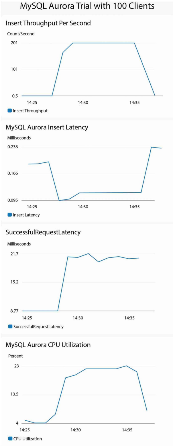
Fig. 9 Aurora MySQL 100 clients trial. This figure shows event counts on the Y-axis in per minute buckets and the X-axis reflects time.
