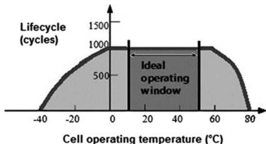
Fig. 3 Lithium-ion battery lifecycle versus temperature diagram
