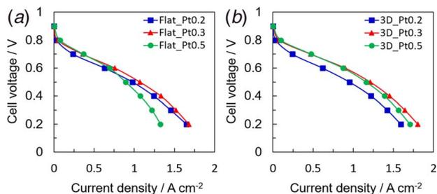
**Fig. 5** Polarization curves of the (a) flat- and (b) 3D-structured CCLs at Pt loadings of 0.2, 0.3, and 0.5 mg/cm<sup>2</sup>
