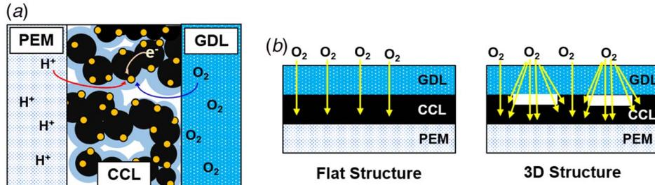
Fig. 1 Schematic of (a) the cathode side and (b) the two CCL structural designs
