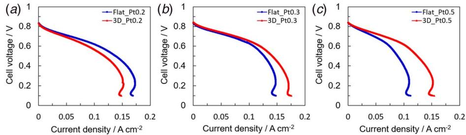
**Fig. 9** Limiting current densities of the two structures at Pt loadings of (a) 0.2, (b) 0.3, and (c) 0.5 mg/cm<sup>2</sup>
