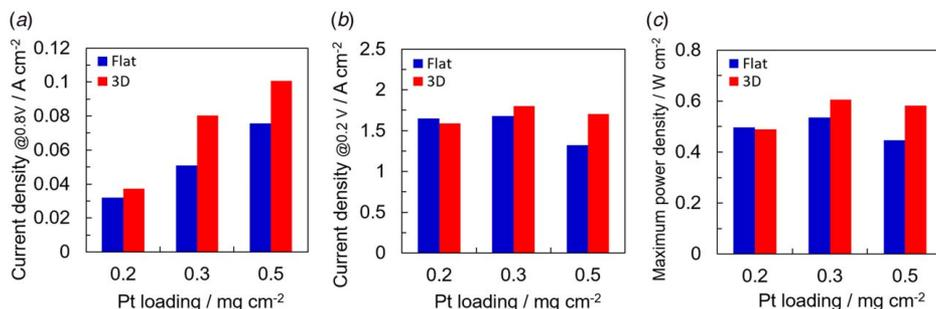
**Fig. 7** Performances of the flat and 3D CCLs at (a) 0.8 V and (b) 0.2 V; and (c) maximum power densities of the two structures at various Pt loadings
