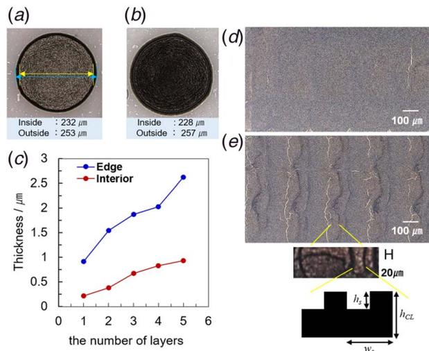
**Fig. 4 The images of the (a) first and (b) fifth printed layers on the Nafion film. (c) The thickness of the CCL as a function of the number of layers. Images of the (d) flat and (e) 3D structures.**
