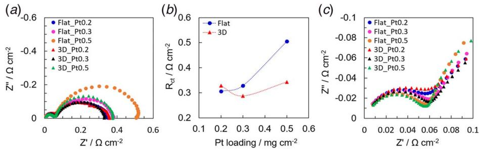
**Fig. 8** (a) Impedance spectra at 0.6 V of the flat and 3D CCLs and (b) charge-transfer resistances of the CCLs at varying Pt loadings. (c) Enlarged impedance spectra of the CCLs over an impedance range of 0–0.1
