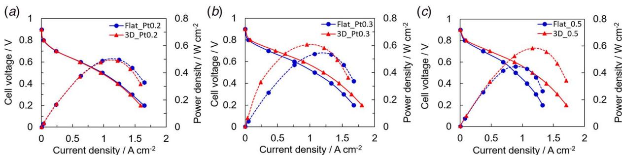
**Fig. 6** Polarization curves and power densities of the 3D- and flat-structured CCLs at Pt loadings of (a) 0.2, (b) 0.3, and (c) 0.5 mg/cm<sup>2</sup>
