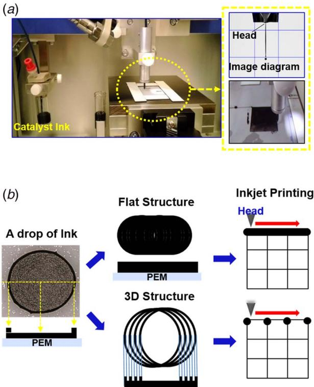
**Fig. 3 Real images of (a) inkjet printing and (b) patterning of the CCL structures**
