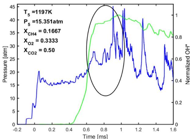
**Fig. 4** Pressure and emission traces for the 50% CO<sub>2</sub>-diluted mixture shown with a circled region of ignition
