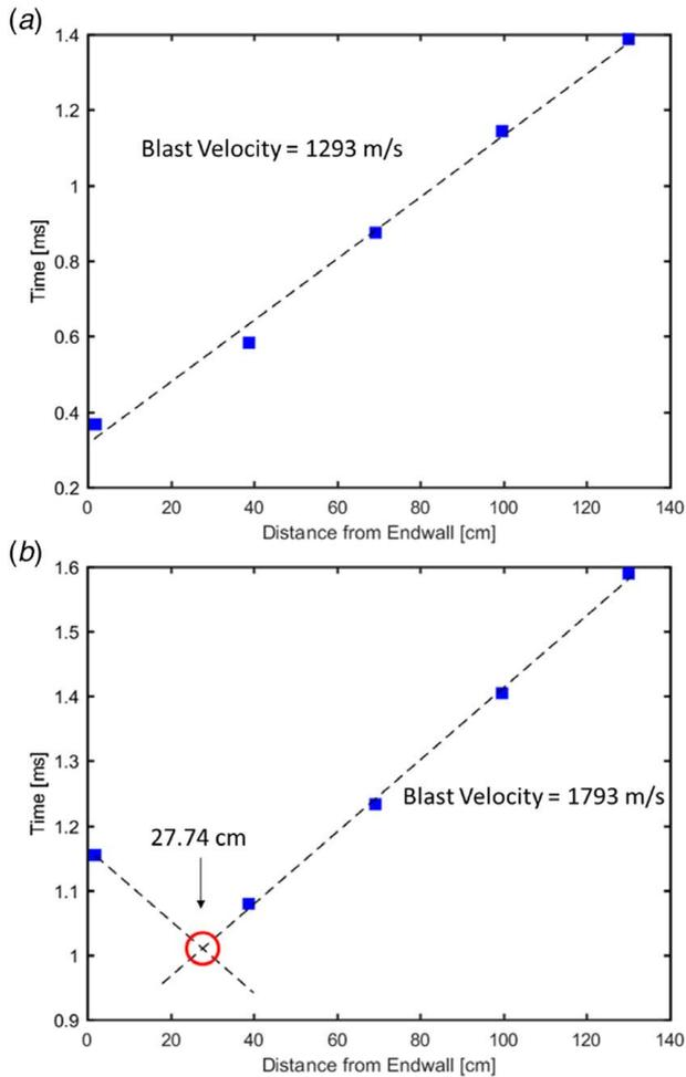
**Fig. 6 Experimental detonation maps for (a) a homogeneous ignition event from the CO<sub>2</sub>-diluted mixture and (b) an inhomogeneous ignition event from the N<sub>2</sub>-diluted mixture; blast location is marked by an open red circle. Blast velocities and location are shown.**
