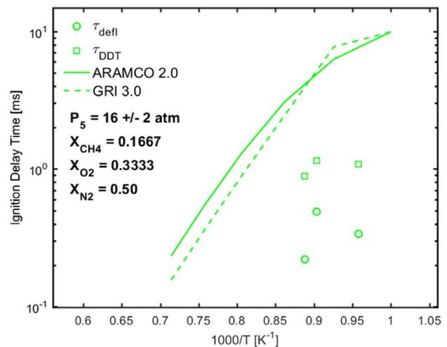
**Fig. 8 Experimental definitions of ignition delay times compared to model predictions using chemkin-pro of the N<sub>2</sub>-diluted mixture. Inhomogeneous events are indicated with open circles and squares.**
