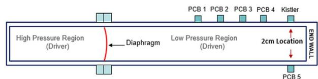
Fig. 1 Schematic of the shock tube facility indicating positions of pressure transducers and test section location
