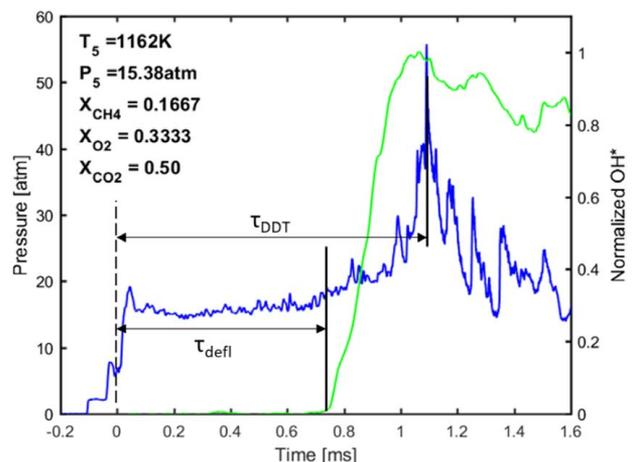
**Fig. 3 Typical experimental pressure and emission traces with labeled definitions of ignition for the 50% CO<sub>2</sub>-diluted mixture**
