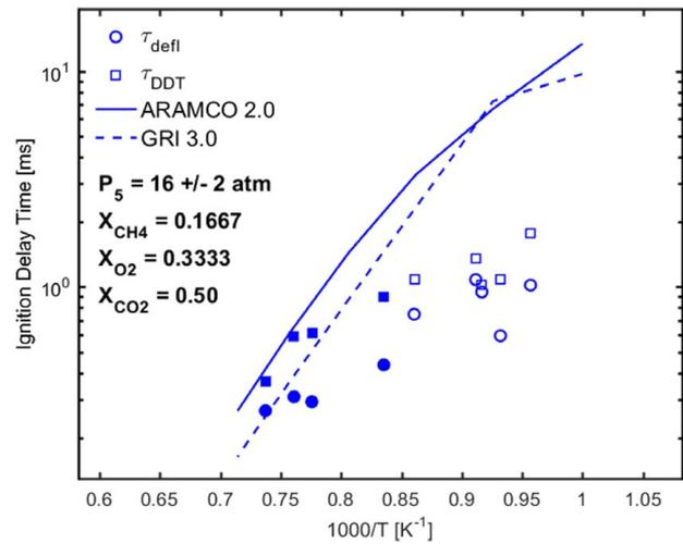
**Fig. 7 Experimental definitions of ignition delay times compared to model predictions using chemkin-pro of the CO<sub>2</sub>-diluted mixture. Homogeneous events are indicated with filled markers.**
