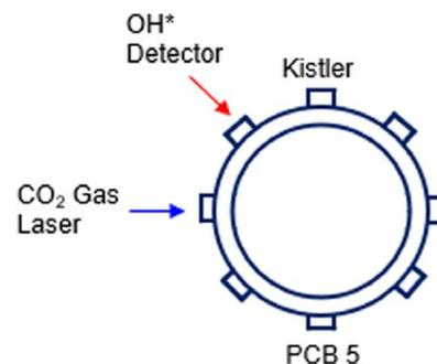
Fig. 2 Schematic showing circumferential positions of various diagnostics used (note this is in plane at the 2-cm location)
