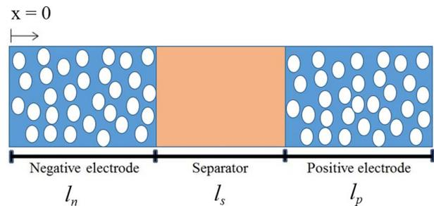
Fig. 1 Schematic of a P2D lithium-ion battery model
