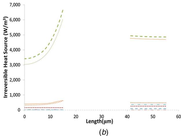
**Fig. 9 (a) Irreversible heat generation in a thick electrode and (b) irreversible heat generation in a thin electrode during 1 C discharge and 5 C charge for distinct combinations of particle sizes. Legend shown in (a) applies to both plots**
