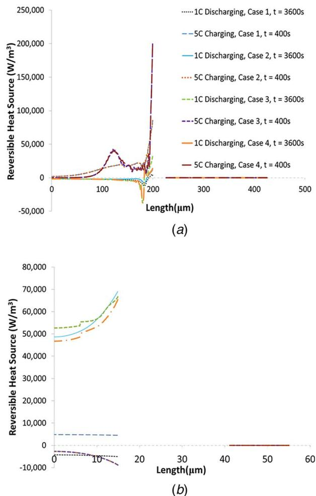
**Fig. 8 (a) Reversible in a thick electrode and (b) reversible heat generation in a thin electrode during 1 C discharge and 5 C charge for distinct combinations of particle sizes. Legend shown in (a) applies to both plots**
