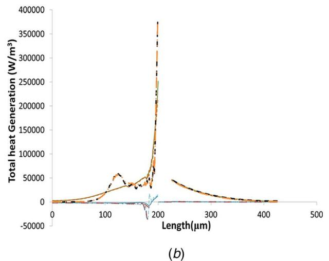
**Fig. 10 (a) Total heat generation in a thin electrode during 1 C discharge and 5 C charge compared with (b) total heat generation in a thick electrode for distinct combinations of particle sizes**
