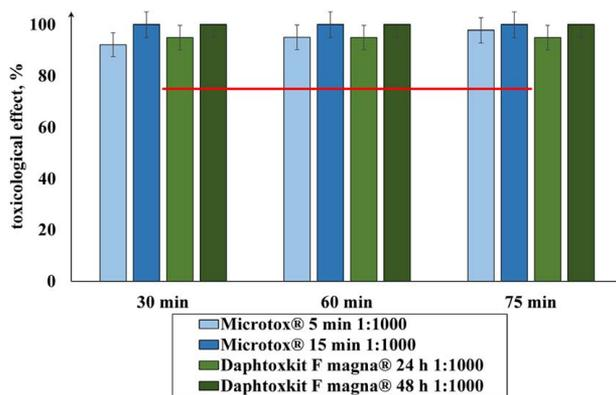
**Fig. 10** The results of the toxicity tests with the limit, marked in red, above which samples are highly toxic (legend: the test name, the test time, and the sample dilution ratio)
