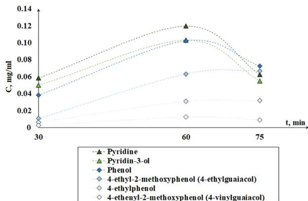
**Fig. 9** The results of the quantitative analysis of some of the pyridine and phenolic contents in the condensables from wheat-rye chaff torrefaction (the measurement errors do not exceed 2.5%)
