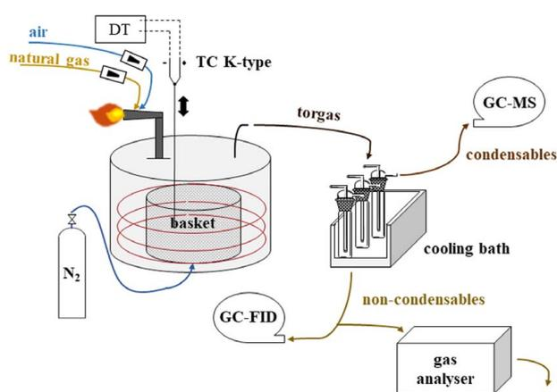
**Fig. 2** A general scheme of the test rig (DT, digital thermometer; TC, thermocouple; and GC-FID, gas chromatograph with flame ionization detector) [28]
