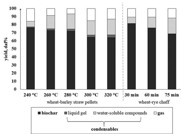
Fig. 3 Torrefaction product yields calculated in reference to the initial feedstock mass in a dry ash-free state
