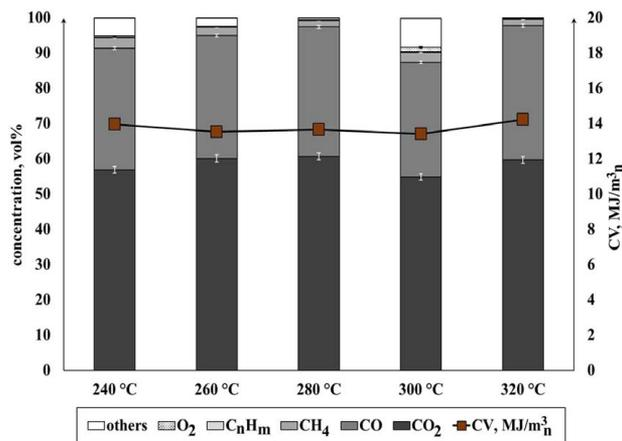
Fig. 4 Average compositions of noncondensables from the wheat–barley pellet (CV, calorific value)
