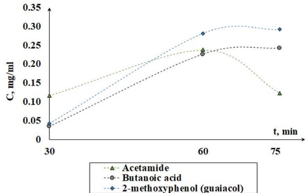
Fig. 8 The results of the quantitative analysis of acetamide, butanoic acid, and guaiacol contents in the condensables from wheat-rye chaff torrefaction (the measurement errors do not exceed 1.45%)
