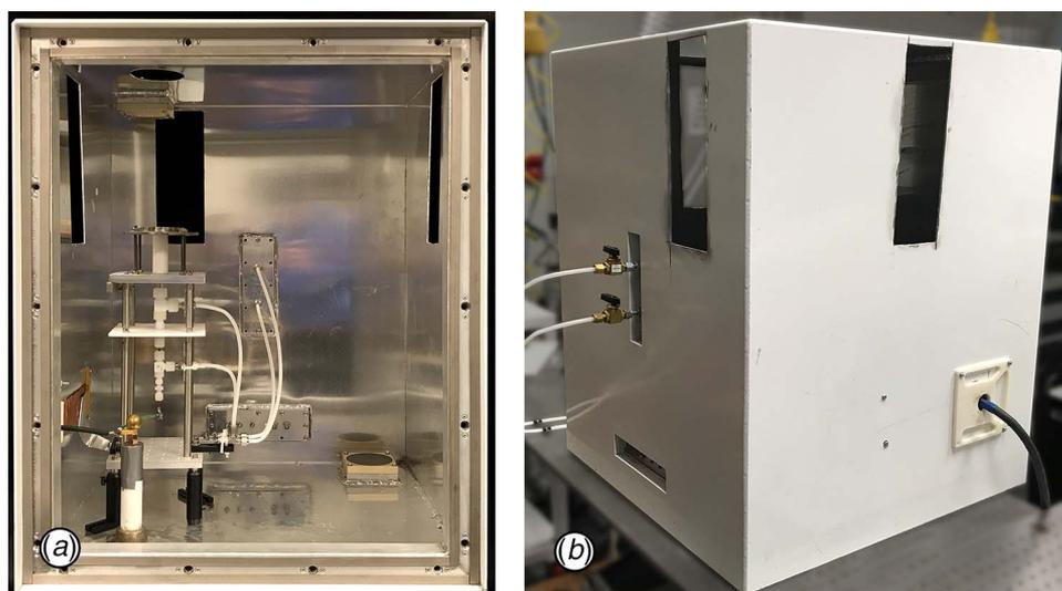
**Fig. 3 Faraday cage (a) front-view with the lid opened and (b) side-view with the lid closed**
