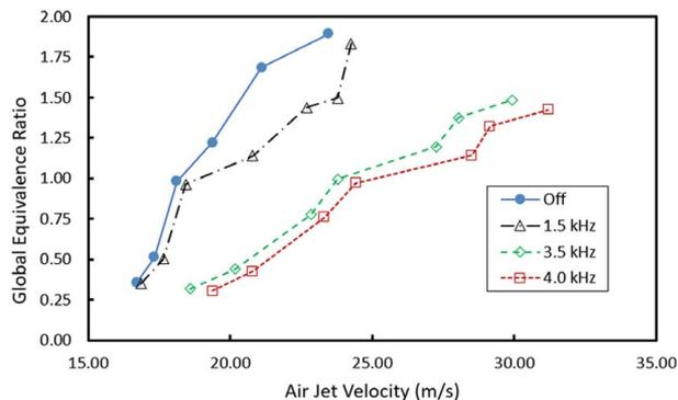
**Fig. 7** Flame extinction conditions in different flow condition by increasing air flowrate at different plasma frequencies
