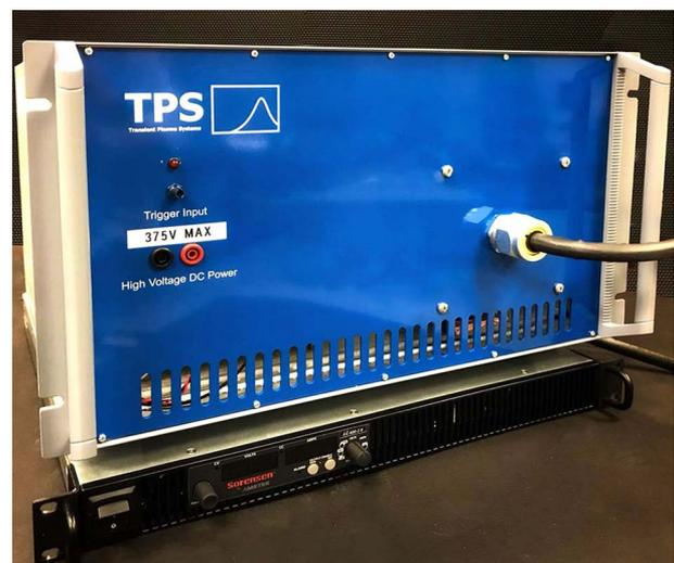
Fig. 2 SSPG-20x nanosecond pulse generator and XG600 dc power supply
