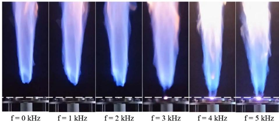
Fig. 5 Effect of RNP discharge frequency on flame stability at different discharge frequencies
