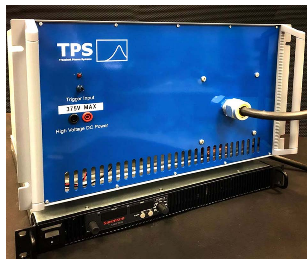
Fig. 2 SSPG-20x nanosecond pulse generator and XG600 dc power supply
