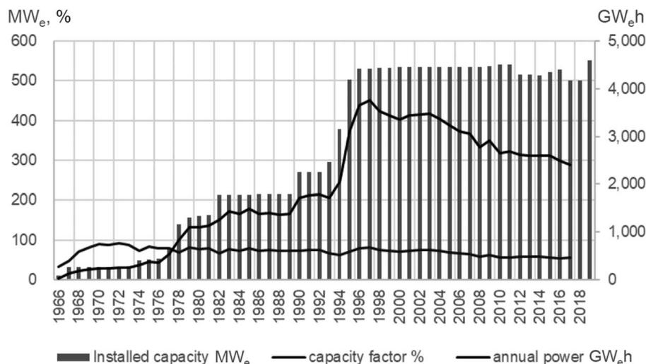
Fig. 1 Geothermal power in Japan: total installed capacity (columns), power generated (darker line), and capacity factor (lighter line) [2]
