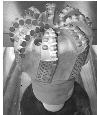
**Fig. 5 Fabricated PDC bit [8]**
