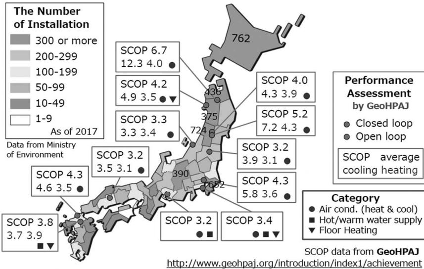
**Fig. 8** The number of GSHP installation in each prefecture in Japan [5] and measured system-COP at several systems [13]
