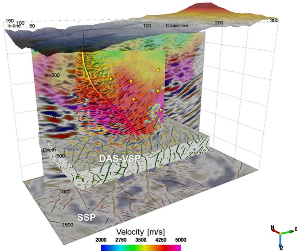
**Fig. 4 Comparison of DAS-VSP and SSP survey results for data obtained at Ogiri geothermal field, Kagoshima [8]**
