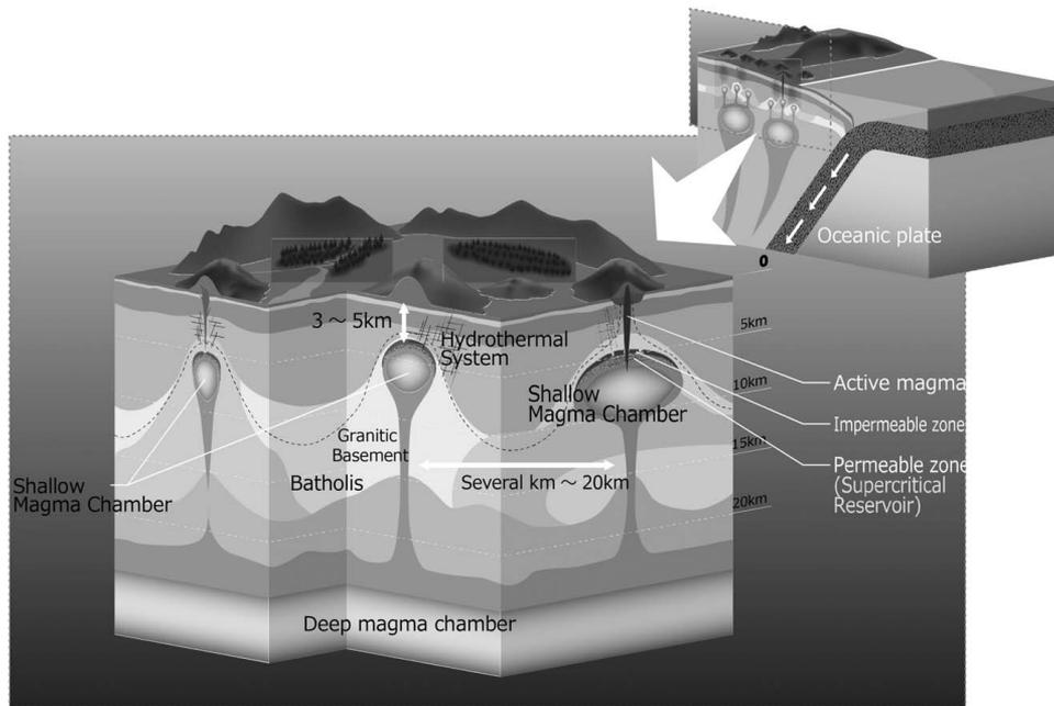
Fig. 6 Conceptual model of supercritical geothermal system in northeast Japan [12]
