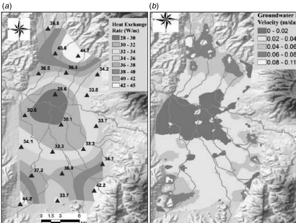
**Fig. 9** An example of suitability map: (a) distribution of sustainable heat exchange rate and (b) distribution of flowing velocity of groundwater [14]
