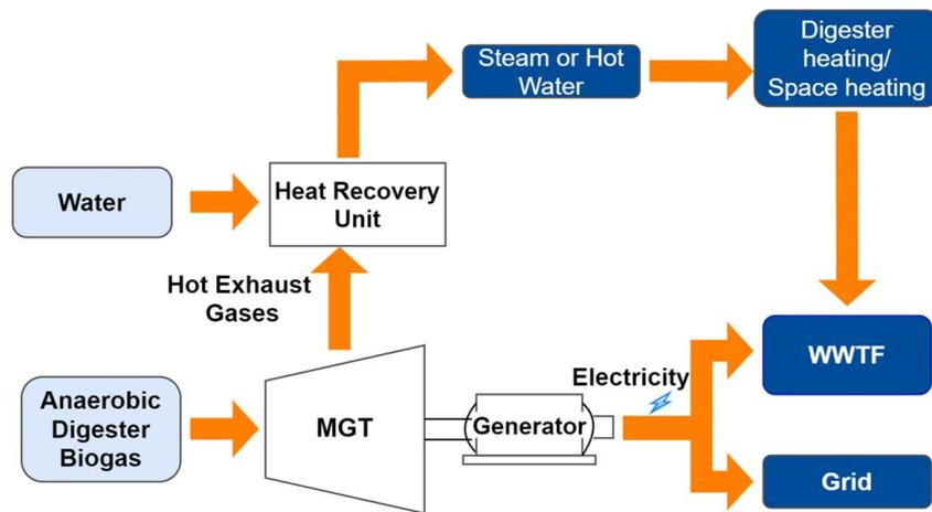
Fig. 3 Typical cogeneration system at WWTP [17]
