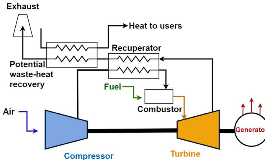
Fig. 2 Microturbine working principle [16]
