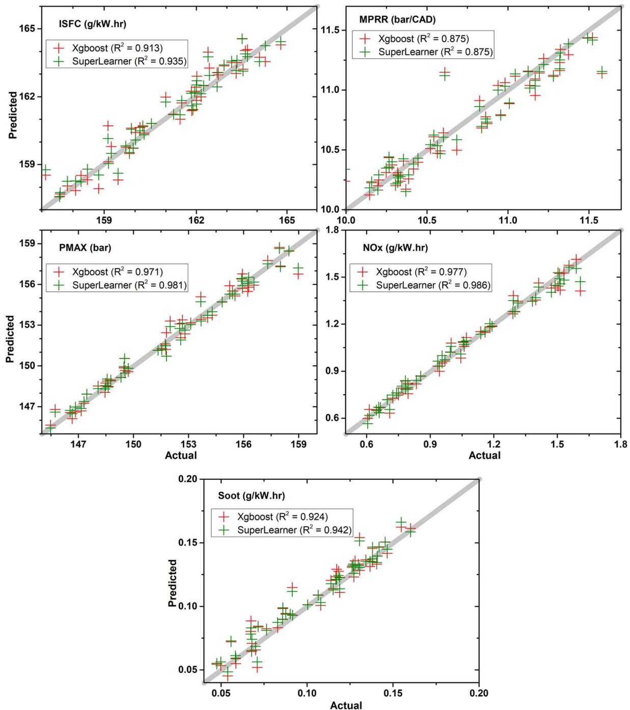
**Fig. 8 Comparison between predicted and actual CFD results of  $\text{NO}_x$  and Soot emissions, fuel consumption (ISFC), maximum pressure (Pmax), and MPRR for 51 testing designs**
