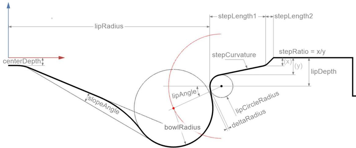
Fig. 6 Piston bowl profile with design parameters
