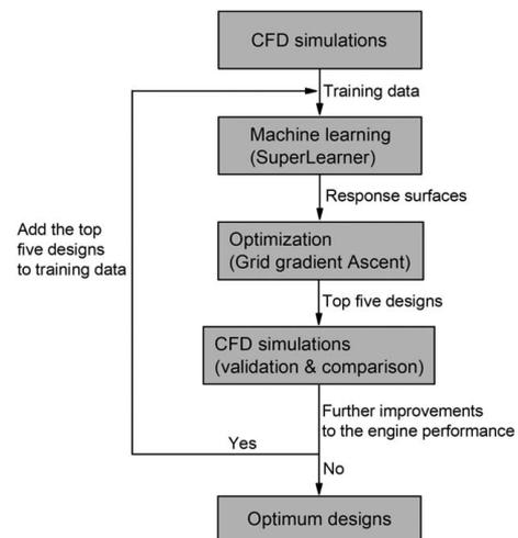
**Fig. 11 ML-GGA piston bowl geometry optimization scheme**
