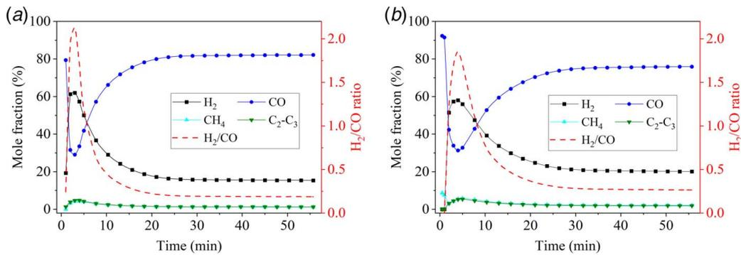
**Fig. 6** Mole fractions of gas components in accumulated syngas gas yield from (a) non-catalytic and (b) catalytic gasification of PS
