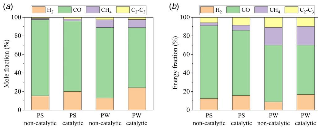
**Fig. 8 (a) Mole fractions and (b) energy fractions of gas components in accumulated syngas yield over 56 min from gasification of PS and PW under non-catalytic and catalytic conditions**
