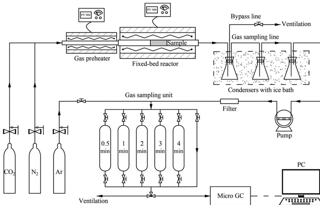
**Fig. 2** Schematic diagram of the fixed-bed reactor system
