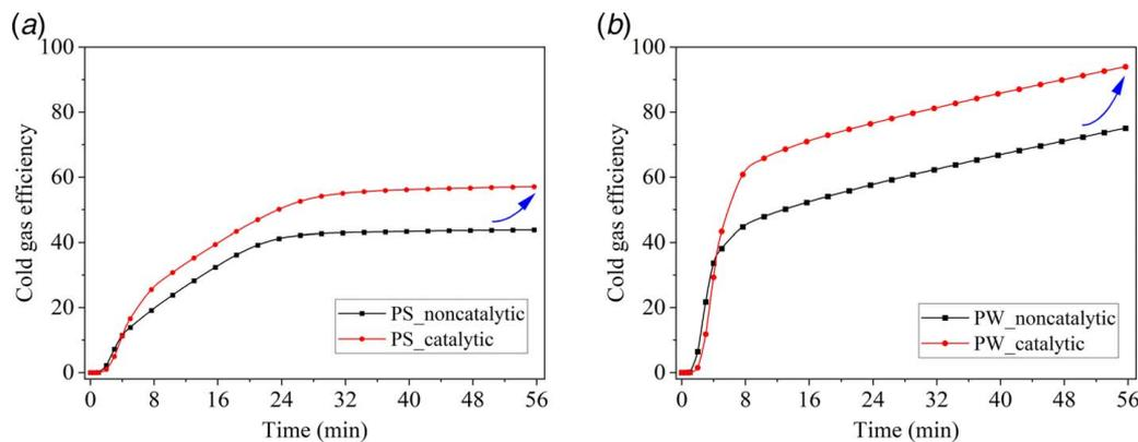
**Fig. 9 Comparison of cold gas efficiency from gasification of (a) PS and (b) PW under non-catalytic and catalytic conditions**
