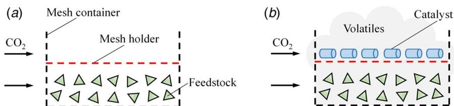
**Fig. 1 Schematic diagram of (a) non-catalytic and (b) quasi-in situ catalytic methods**
