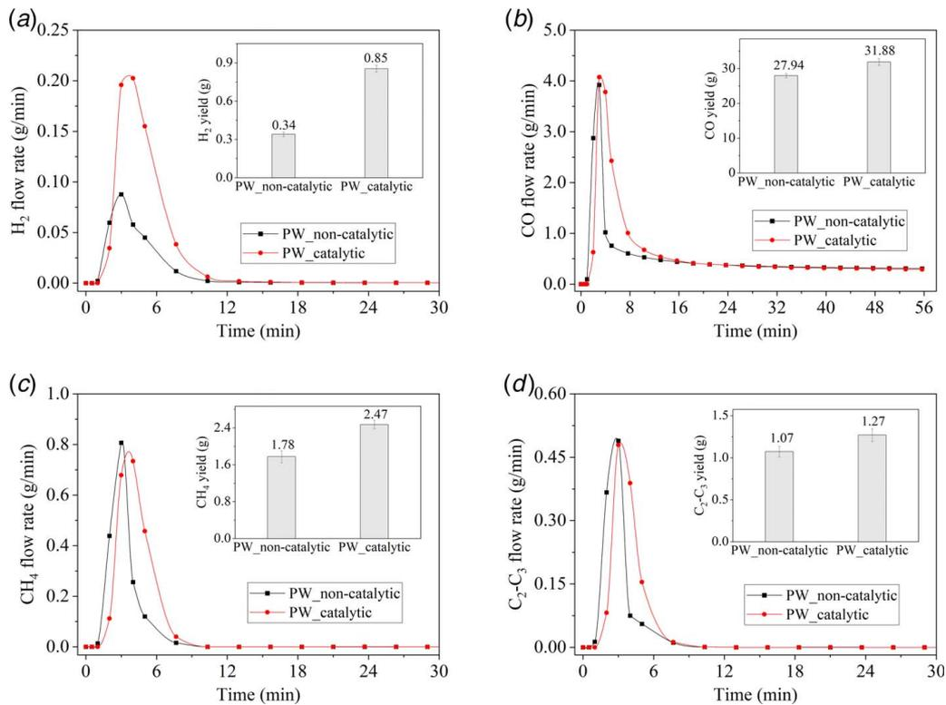
**Fig. 4 Evolution and cumulative yields of (a) H<sub>2</sub>, (b) CO, (c) CH<sub>4</sub>, and (d) C<sub>2</sub>-C<sub>3</sub> from non-catalytic and catalytic gasification of PW**
