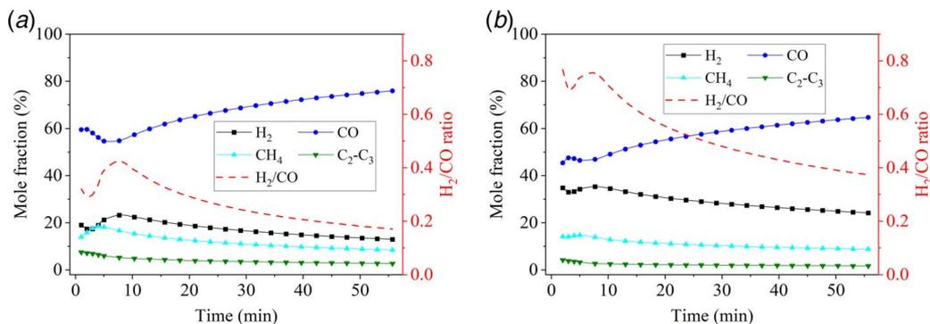
**Fig. 7** Mole fractions of gas components in accumulated syngas gas yield from (a) non-catalytic and (b) catalytic gasification of PW
