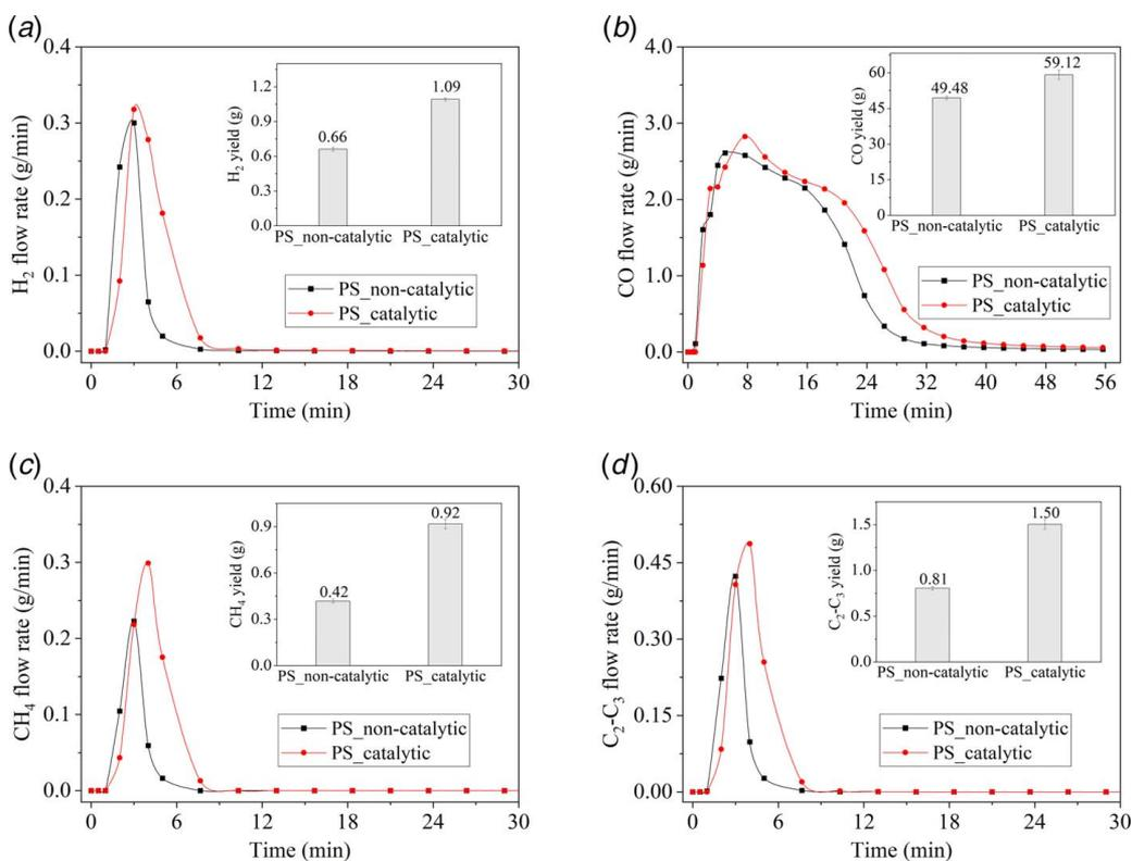
**Fig. 3** Evolution and cumulative yields of (a) H<sub>2</sub>, (b) CO, (c) CH<sub>4</sub>, and (d) C<sub>2</sub>-C<sub>3</sub> from non-catalytic and catalytic gasification of PS
