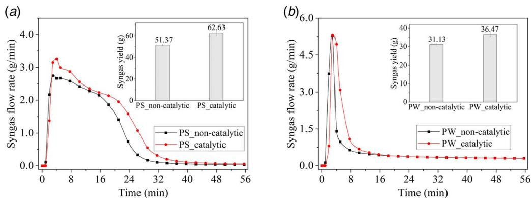
**Fig. 5 Evolution and cumulative yields of syngas from gasification of (a) PS and (b) PW under non-catalytic and catalytic conditions**
