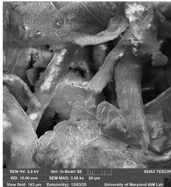
Fig. 7 SEM images of (a) the raw cellulose and (b) raw cellulose (magnified) used for the SCC tests
