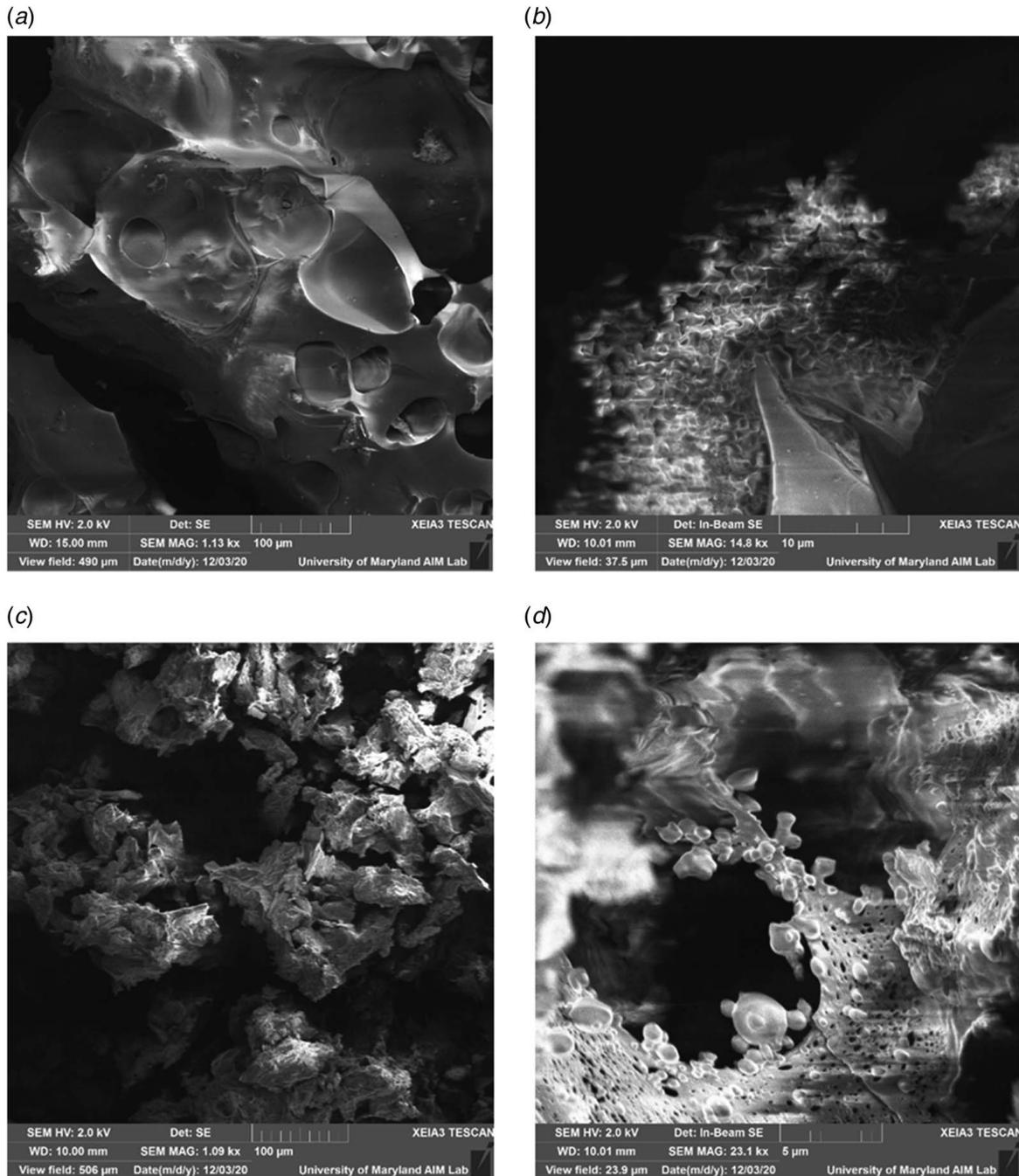
**Fig. 8** SEM images of the chars obtained from SCC of cellulose at (a) 623 K for 2 h of residence time, (b) 623 K for 2 h (magnified), (c) 623 K for 5 h of residence time, and (d) 623 K for 5 h (magnified)
