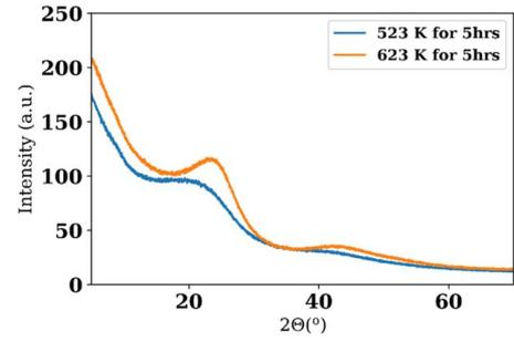
Fig. 5 Powder XRD patterns of selected char samples obtained from SCC of cellulose at 523 and 623 K temperature at 5 h residence time
