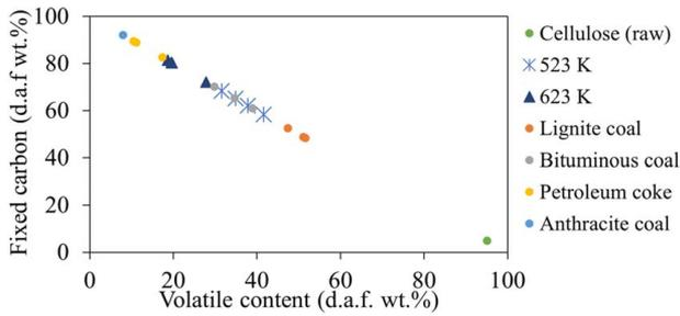
**Fig. 1 Comparison of extents of carbonization from SCC chars with cellulose and different coals (d.a.f: dry ash free) [64]**
