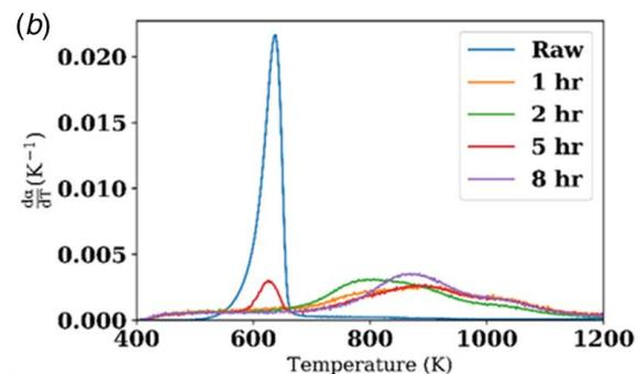
**Fig. 2 TG behavior of SCC chars obtained at (a) 523 K and (b) 623 K temperatures and different residence times (and also raw cellulose)**
