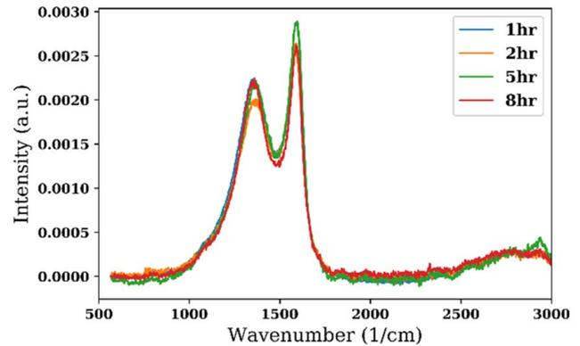
**Fig. 3 Intensity versus wavenumber from Raman spectra of SCC chars obtained at 523 K temperature and different residence times**
