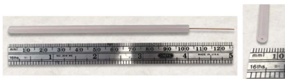
Fig. 3 Example wire sample with (left) core length of 125 mm (4.9 in.) and LDPE insulation length of 100 mm (3.9 in.) and (right) 0.64 mm (0.025 in.) diameter copper core and LDPE insulation with 4 mm (0.16 in.) outer diameter [23]
