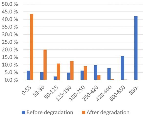
**Fig. 2 PSD of CaCO<sub>3</sub> with  $D_{50}$  approximately at 600  $\mu\text{m}$  before and after degradation**
