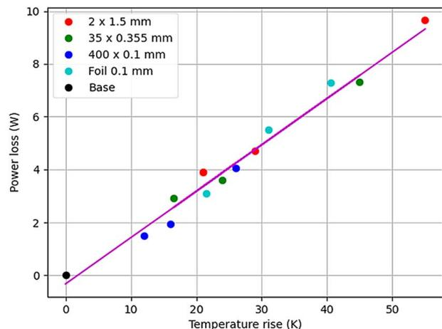
**Fig. 5 Calibration characteristic of the calorimetric chamber**
