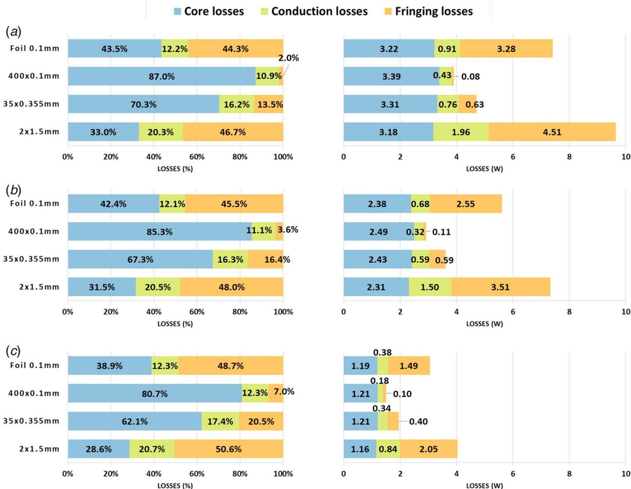
**Fig. 6** Decomposed power losses of the inductors for three cases: (a) 4A root-mean-square (RMS), (b) 3.5A RMS, and (c) 2.6A RMS
