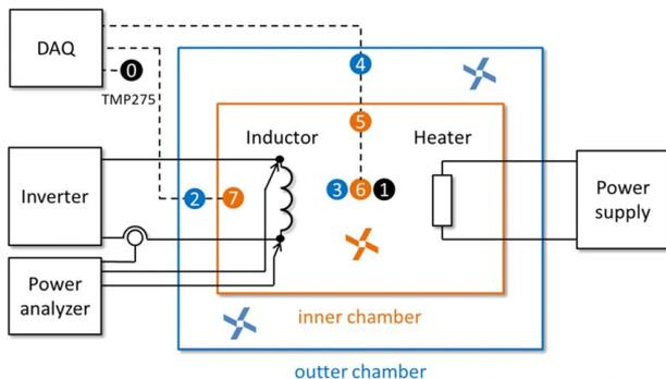
**Fig. 2** Diagram of the system for calorimetric measurement
