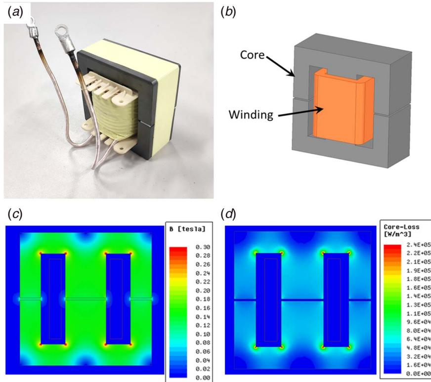
**Fig. 4 FEM simulation: (a) assembled inductor to model, (b) geometry setup, (c) magnetic flux density distribution, and (d) core power loss distribution**
