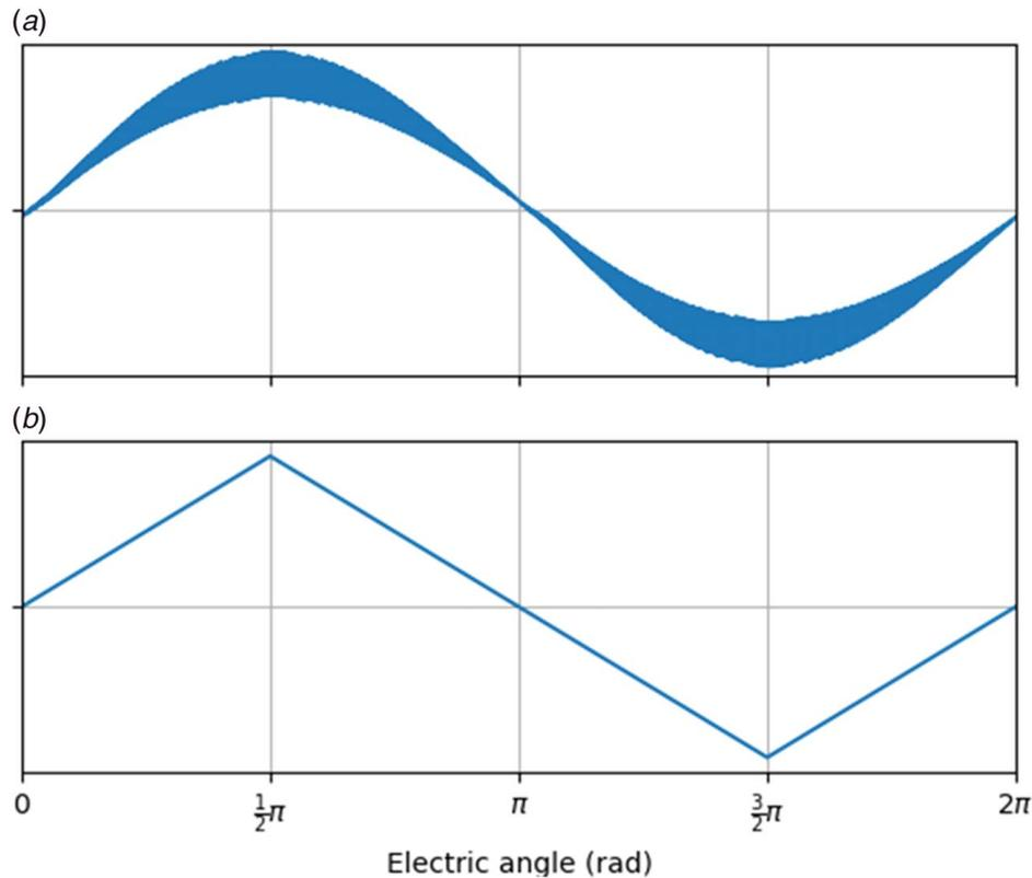
**Fig. 1** Example waveforms typical for power electronic devices: (a) sinusoidal with high-frequency ripple and (b) triangular waveform
