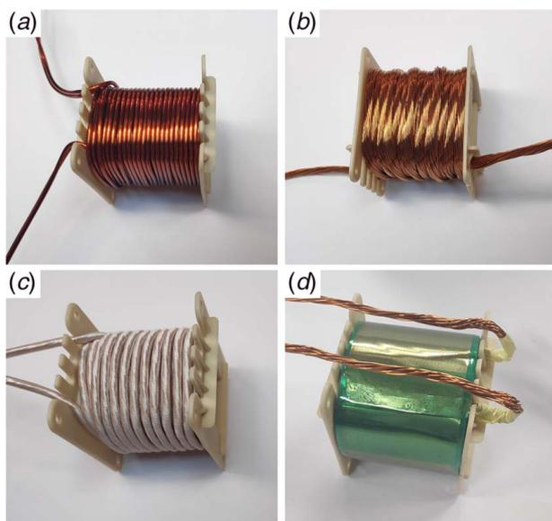
**Fig. 3** Windings used in research (a)  $2 \times 1.5$  mm, (b)  $35 \times 0.355$  mm, (c)  $400 \times 0.1$  mm, and (d) foil  $0.1 \times 34$  mm
