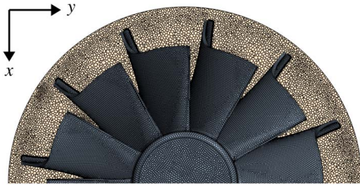
Fig. 5 Detailed view of the mesh inside the rotor at a section in the x - y plane
