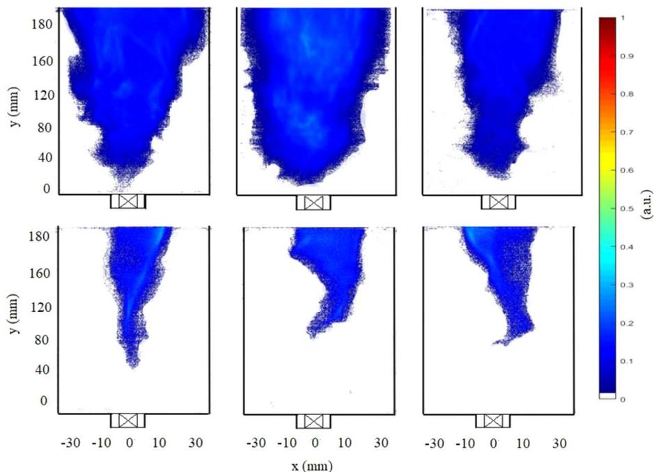
**Fig. 4** Instantaneous chemiluminescence images near to blowoff. Top row at  $\phi_{LBO} + 0.06$ , and bottom row at  $\phi_{LBO} + 0.02$  using propane fuel (at heat release intensities of  $9.53 \text{ MW/m}^3\text{-atm}$ ).
