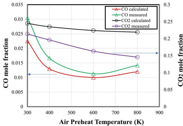
**Fig. 9 CO and CO<sub>2</sub> concentrations near blowoff ( $\phi_{LBO} + 0.02$ ) at different air preheat temperatures**
