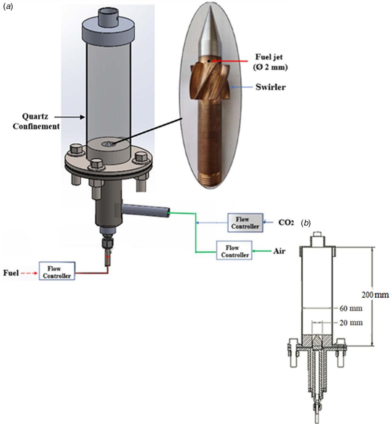
Fig. 1 (a) Sketch of the model experimental swirl combustor (left) and the swirler location in air passageway of the burner (right). (b) Cross-sectional view of the burner.
