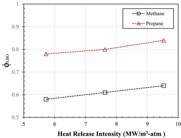
**Fig. 2** Lean blowoff equivalence ratio at different heat release intensities in distributed combustion using propane and methane fuels
