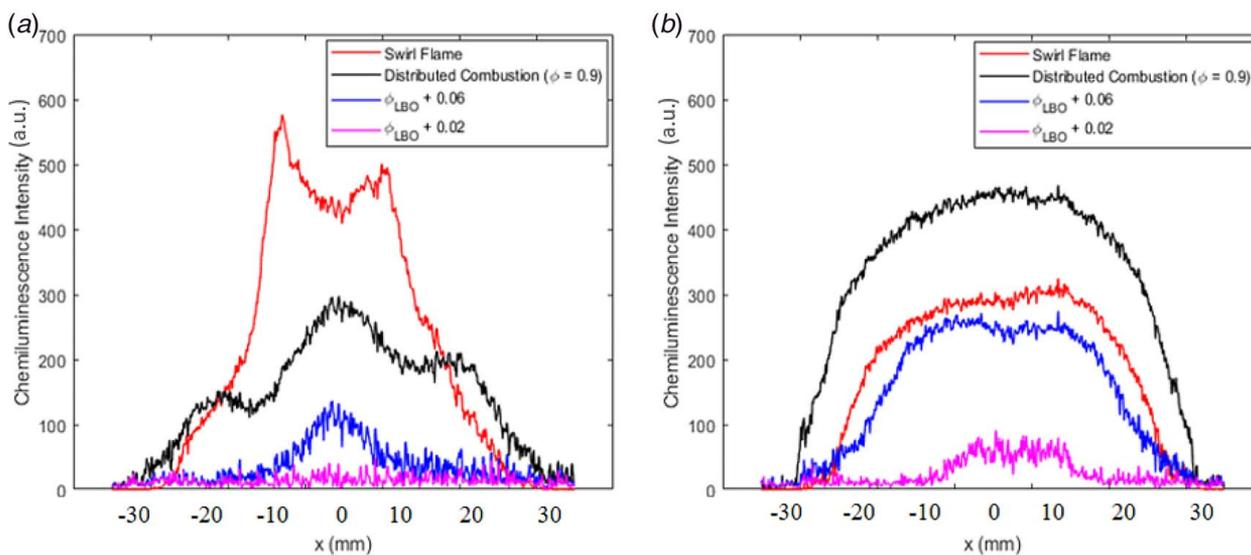
**Fig. 5** Radial distribution of chemiluminescence intensity at (a) near-burner exit flowfield (at  $y = 25 \text{ mm}$ ) and (b) farther away flowfield (at  $y = 135 \text{ mm}$ ) using propane fuel (at heat release intensities of  $9.53 \text{ MW/m}^3\text{-atm}$ )
