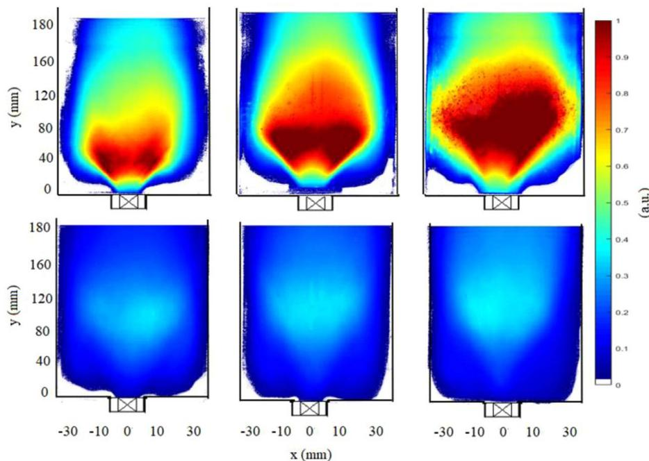
**Fig. 3** Average of 500 chemiluminescence images of stable swirl combustion (at  $\phi = 0.9$ ) (top row) and distributed combustion (bottom row) at heat release intensities of 5.72, 7.63, and  $9.53 \text{ MW/m}^3\text{-atm}$  using propane fuel
