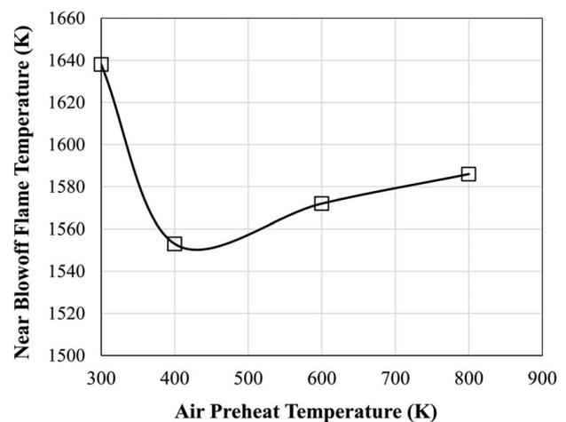
**Fig. 8** Adiabatic flame temperature ( $T_{ad}$ ) near blowoff ( $\phi_{LBO} + 0.02$ ) of methane flame for three different air preheat temperatures
