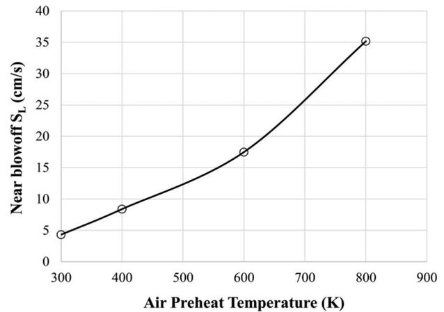
**Fig. 7** Laminar flame speed ( $S_L$ ) near blowoff ( $\phi_{LBO} + 0.02$ ) for methane fuel at different air preheat temperatures
