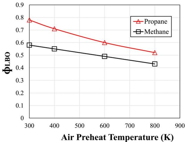
**Fig. 6** Lean blowoff equivalence ratio of propane and methane flames (at  $5.72 \text{ MW/m}^3\text{-atm}$  heat release intensity) with  $\text{CO}_2$  dilution at different air preheat temperatures
