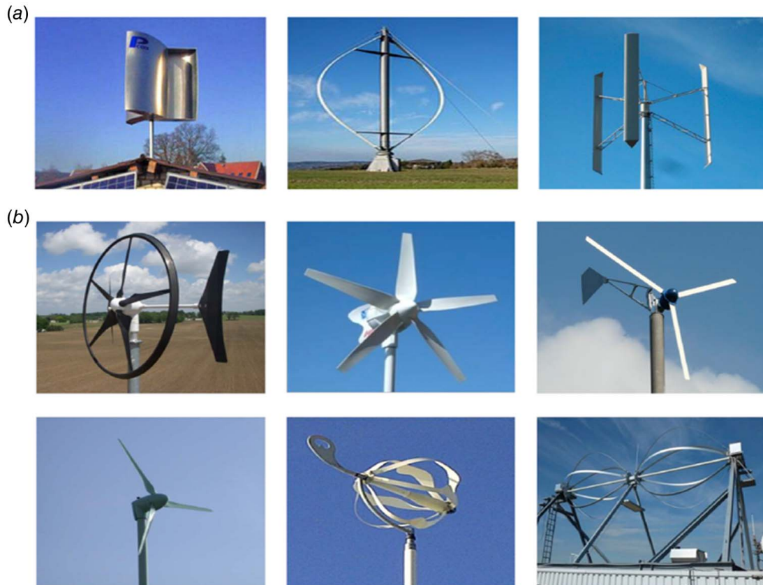
Fig. 2 Taxonomy of (a) vertical axis turbines and (b) horizontal axis turbines, Ref. [22]
